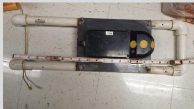
Example of Sontek SW acoustic Doppler current profiler (ADCP) and mounting bracket used for installation inside the downstream ends of pipes 2 and 6, as counted from the north end of S-152.
